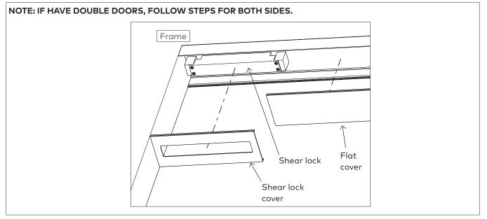
NOTE: Shear lock is pre-installed into header tube.
